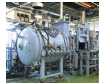
(Next-generation) Decompressed carburizing furnace
