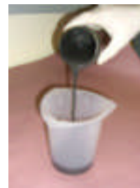
Conductive ink made with silver nano-particles
